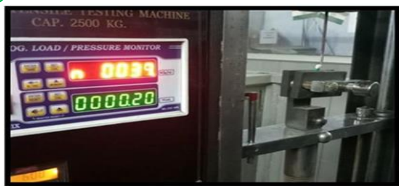
Fig 5: Value obtained in the universal testing machine for shear bond strength.
