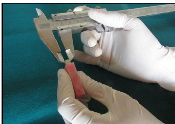
Fig-2 Measuring of specimen with Vernier calliper to produce specimens of 4x4mm 2
