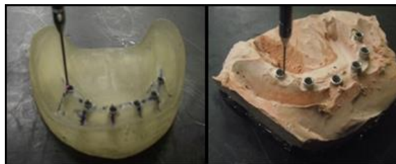
Fig 10: Measurement of acrylic resin model and master cast in X,Y,Z axes by CMM machine.
