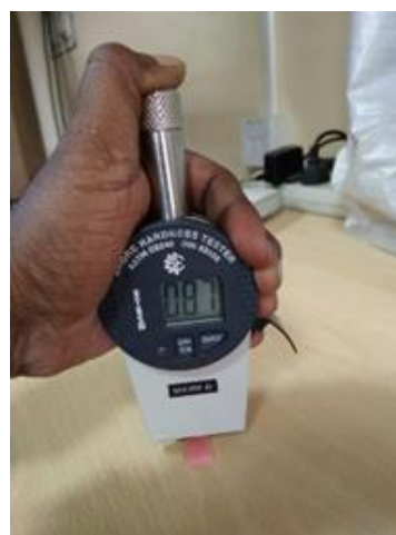
Fig 3: Testing of specimen for surface hardness.
