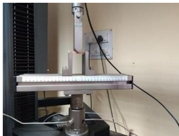
Fig 2: Testing of specimen for flexural strength.
