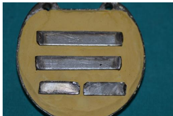
Fig 1: Stainless steel dies invested in dental stone.
