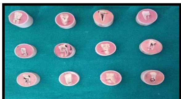
Fig 3b: Acrylic resin block for microhardness analysis for (Smart Burs)
