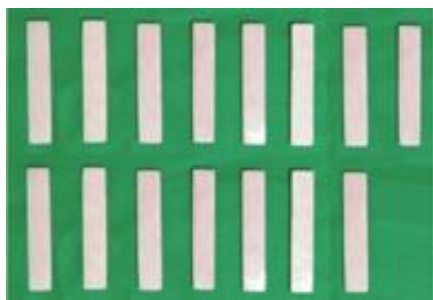
Fig 6: Color plate 6 – Group D Silanized Alumina Nanoparticles Reinforcement
