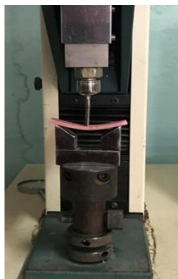
Color plate 8 -Test For Transverse strength under Progress
