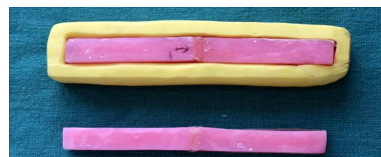
Fig 3: Fabrication of UFI gel p specimen.
