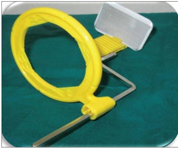
Figure 3: Film holder with gridded intra oral periapical radiograph film
