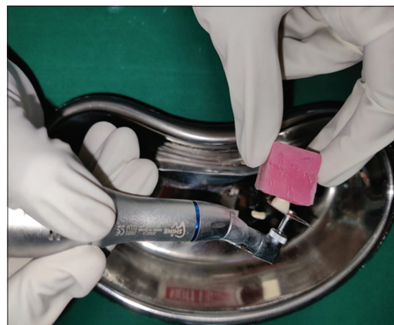
Figure 2: Crown fractured with diamond disc 5 mm from the incisal edge
