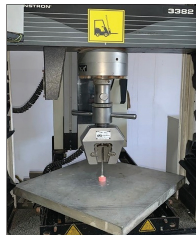
Figure 5: Sample testing for fracture resistance under universal testing machine
