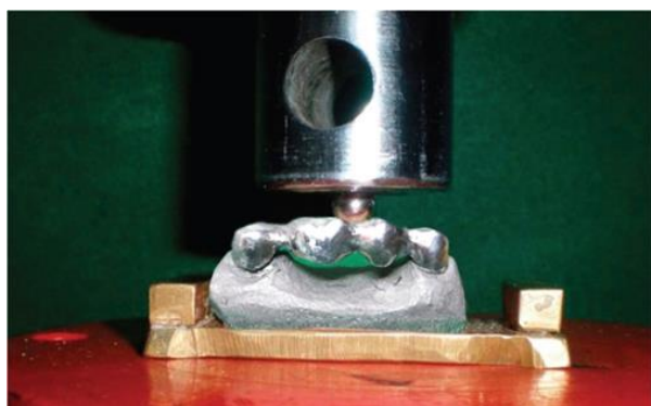
Fig 2: Load Testing Of Group II Samples- NiCr metal framework.
