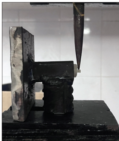
Figure 3: Sample mounted on universal testing machine
