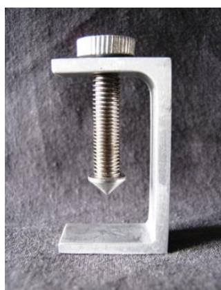
Fig 4: spring loading device.
